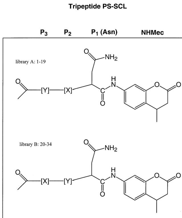
Fig. 2. Tri-peptide-AMC combinatorial positional-scanning library. The library consists of two sublibraries of 361 compounds each (10 wells of 19 compounds). Each library is acylated at the amino terminus, contains asparagine at P1, and is tagged with an AMC fluorophore. X represents a specially addressed amino acid and Y represents an isokinetic mixture of the 1–19 amino acids described previously.
